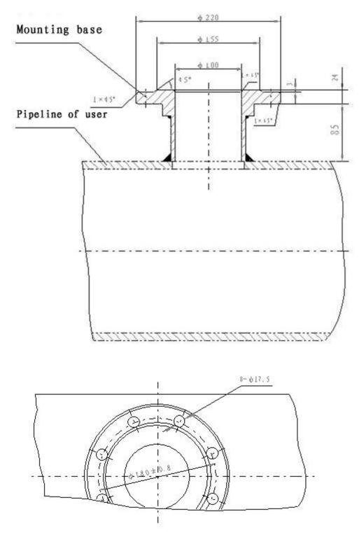
Figure 3 The schematic diagram of the mounting base.
