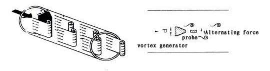
Figure1 The working principle of the vortex-shedding flowmeter
