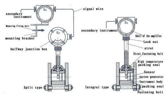
Figure2 The schematic diagram of instrument structure
